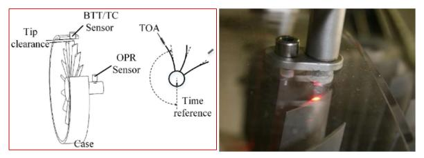
BTT/TC sensor : Blade Tip timing sensor to detect blade passing-by OPR sensor : Once Per Revolution sensor; time reference TOA : time of arrival
