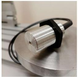
The exposure temperatures are higher than the electronics could withstand. They will therefore cover applications such as automotive turbocharger testing and aeronautical turbomachinery, even if the maximum temperatures are found to be over 1000°C in some cases.
