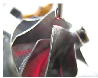
The example above shows a so-called "SLIT" probe, capable of detecting blades or splitters with a thickness of about 1mm on the edge.
