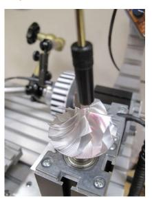
We managed the sensor setting with the potentiometer at the same time as the distance between the blades and the probe. As our tests were carried out at low speeds, we needed to obtain pulses at the passage of the blade with a width sufficient to have a duty cycle of about 80/20 (Figure below). This would allow operators working at higher speeds to obtain a duty cycle closer to 50/50 or even 20/80 in order to provide the acquisition system with incoming signals that are easier to process.
